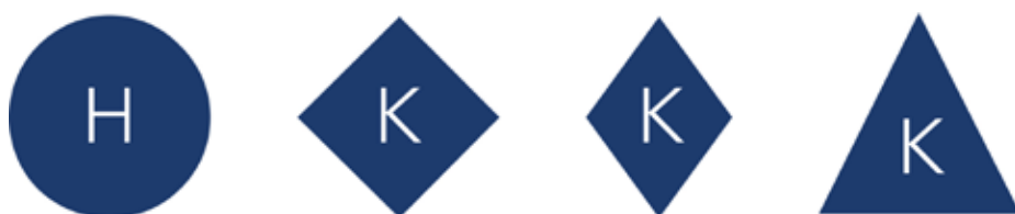
Figure 6. Hedstrom files are round in cross-section; K files, square; K-Flex, rhomboid and K-Flexo files, triangular. The triangular cross-section improves flexibility.
